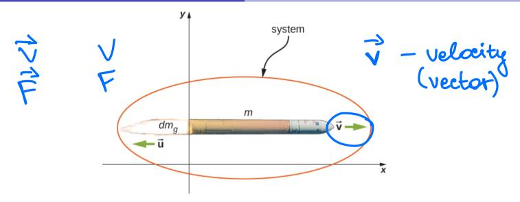
Description: The rocket accelerates to the right due to the expulsion of some of its fuel mass to the left. Conservation of momentum enables us to determine the resulting change of velocity. The mass m is the instantaneous total mass of the rocket (i.e., mass of rocket body plus mass of fuel at that point in time).
